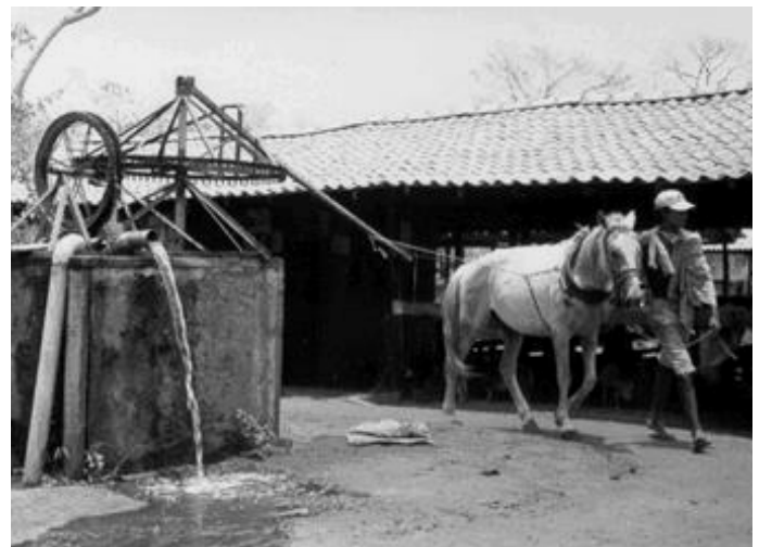
Animal powered Rope Pump
