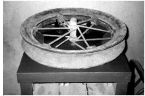
Welding jig for pulley wheel
