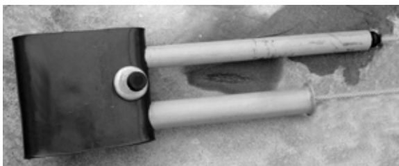
PVC guide box with glass bottle
